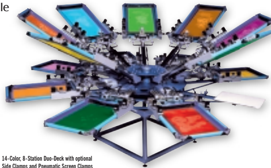
14-Color, 8-Station Duo-Deck with optional Side Clamps and Pneumatic Screen Clamps
